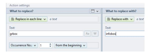
There are various types for the editing of the text (for example, Replace, Insert). These types are called actions. Actions consist mostly of two areas. In one area is defined which part of the text should be edited. The other area is used to define the way in which this part of the text is to be changed or adjusted. Actions can be combined and are applied in the order they occurred. The actions including the filter and sort settings can be saved in a profile.
