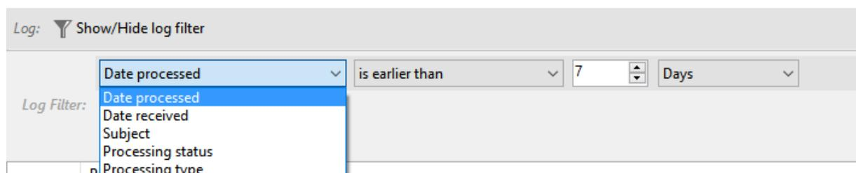
By using the log filter, log entries can be limited. The filter criteria may be, for example, the date of receipt, which is to be limited to a period within the last week. The comparison operator is context-sensitive, that is, he always fits the selected filter criteria. By clicking on the button with the plus or minus symbol, further filters can be added (linked with a logical AND) or the respective filter will be removed.
